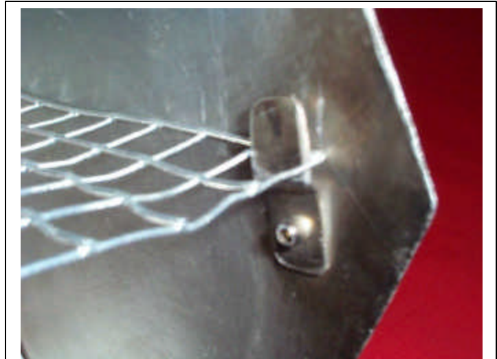
Figure 6 Rack support is located as shown. You may want to round the corners of the rack support or even taper the top portion of the rack support to make it easier for it to go between the wire mesh.
