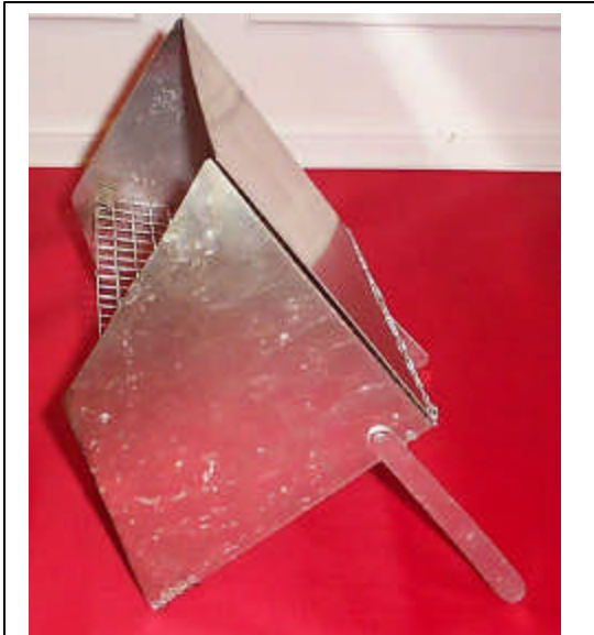
Figure 5 Legs are pop riveted onto the sides as shown. Leg should be able to rotate. Note that pop rivet head is on the leg side not the inside of the oven.
