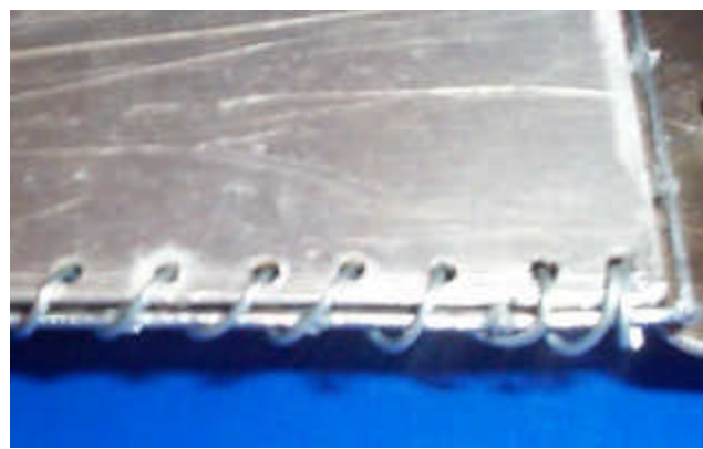
Figure 3 Completed stitching – view looking at the back of the top/bottom hinge. Note the double stitch on the end.
